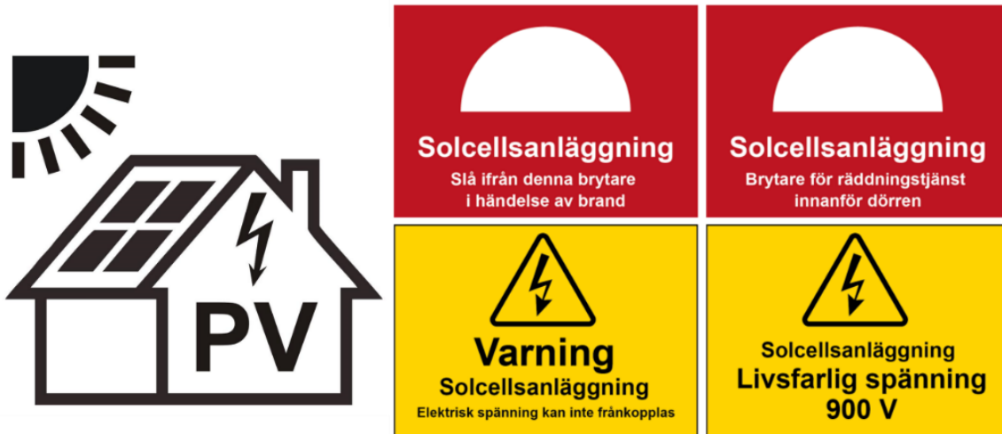
Figure 3. Examples of signage used for photovoltaic installations.
